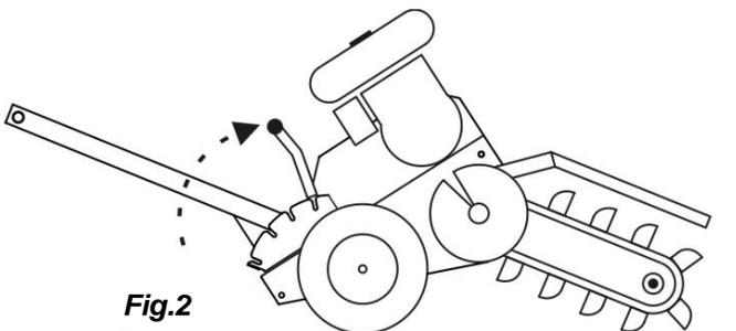
3. Apply downward pressure to the handlebar so the digging chain is not in contact with the ground. Increase the engine speed and hold on to the handlebar with both hands. Slowly relieve the downward pressure on the handlebar allowing the digging chain to penetrate the soil until the chosen depth is reached. **Fig. 3**
