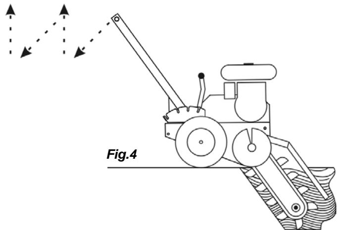
5. Repeat this action until you have finished the job. The wheel lock will aid you in this operation by helping to hold the trencher in position until the next motion is started.
