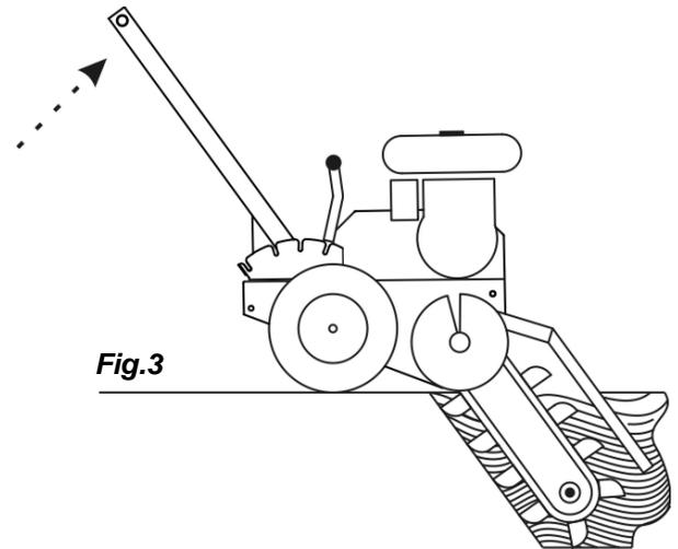
4. Using an intermittent pulling action, pull the trencher toward you 4 to 6 inches then relax your pull, allowing the trencher to again reach the chosen depth. **Fig. 4**
